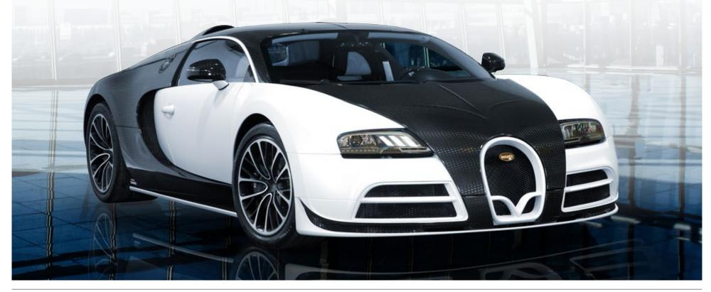
The newly developed side skirts act as a visual and aerodynamic link between the two axles. Larger air outlets on the flanks of the vehicle and at the rear give optimised motor cooling, and together with the new diffuser and the two air intakes, they underline the transition from roof to bonnet on this powerful car design.
