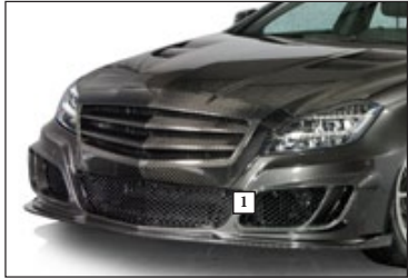
1.1 Front bumper with visible carbon lip, grill and LED DRL ① Only for car without distronic
