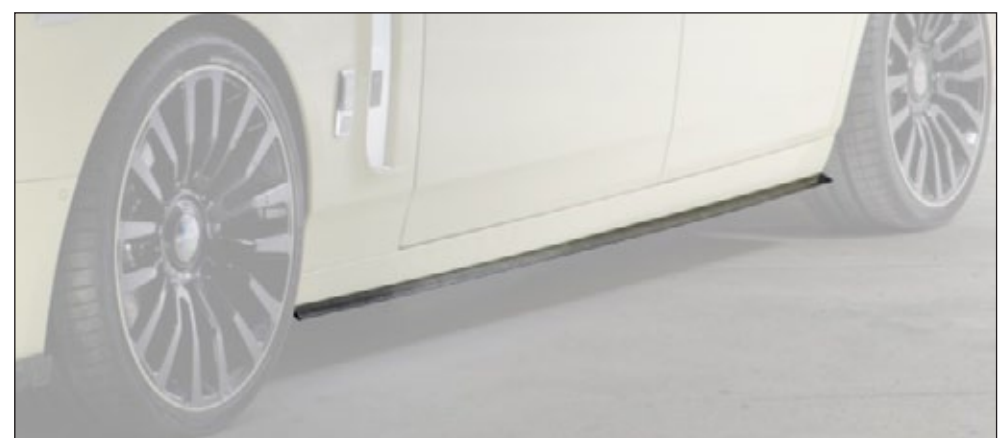
Side skirts lip RR8 595 002 2 parts set - left & right, visible carbon fibre primed without clear coat Side skirts lip EWB RR8 595 012 2 parts set - left & right, for long version visible carbon fibre primed without clear coat,
