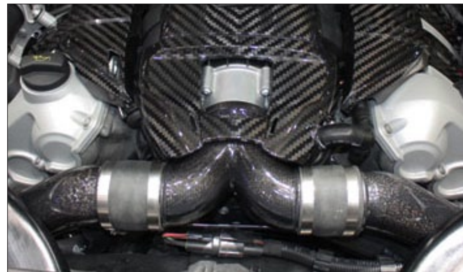
Turbo Upgrade 971 310 02 modified turbochargers, supplementary control unit, set of cables. modifications the engine output rises to an impressive 500 kW / 680 hp (series: 382 kW / 520 hp)
