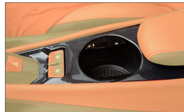
Middle console rear cover F12 363 731 visible carbon fibre primed without clear coat
